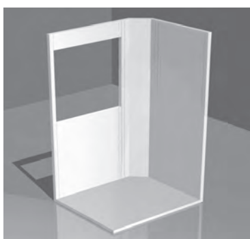
Panels arrive at site complete ready for mounting. Installation is fast due to the interlocking cleat system used to secure the panels.)
