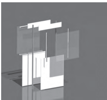
Titan steel panels with bonded composite infill provide great strength and rigidity.)
